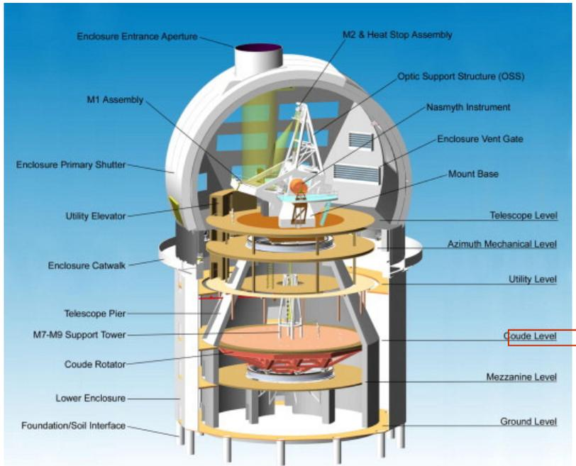
**Advanced Technology Solar Telescope (ATST)** will have a 4 m mirror and capable of observing objects on the Sun that are 30 km across. It is planned to be built atop the Haleakala volcano on the Pacific island of Maui.
