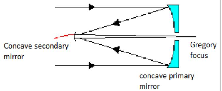
difference to the Cassegrain principle is the use of a concave secondary mirror which produces a real picture (no upside/downs) whereas Laurent Cassegrain (born around 1629 in region of Chartres) used a convex mirror which produces an upside/down or virtual picture of the object.
