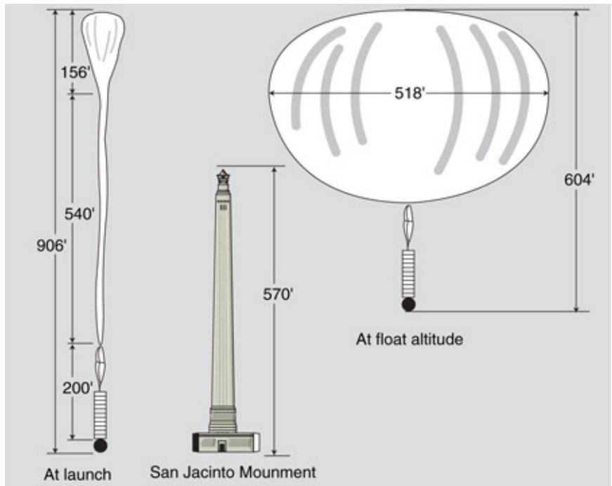
An example how large stratospheric balloons are. The balloon is barely filled at the launch but will be completely expanded when it reaches its destined altitude.
