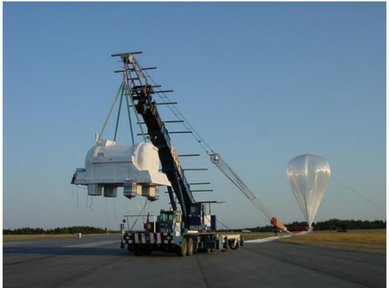
Upper picture: Filling of the balloon with helium or hydrogen. Left picture: The telescope is suspended on a crane. In the background the parachute (orange) and the balloon.
