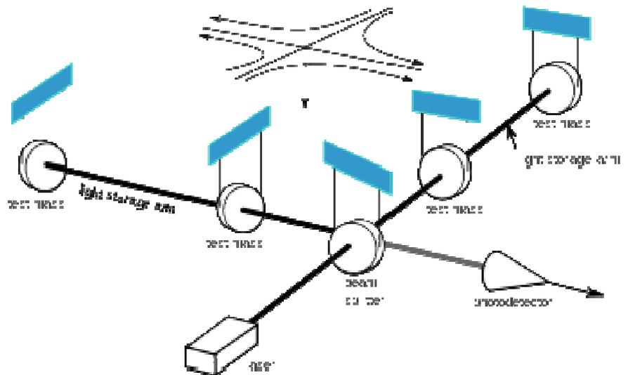
A schematic diagram of a laser interferometer. Source Wikipedia
