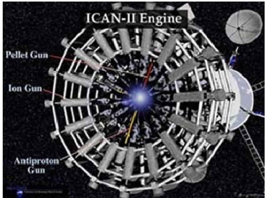
"The ICAN-II (ion compressed antimatter nuclear II) spacecraft designed at Penn State would use the ACMF engine and only 140 nanograms of antimatter for a manned 30-day crossing to Mars".
