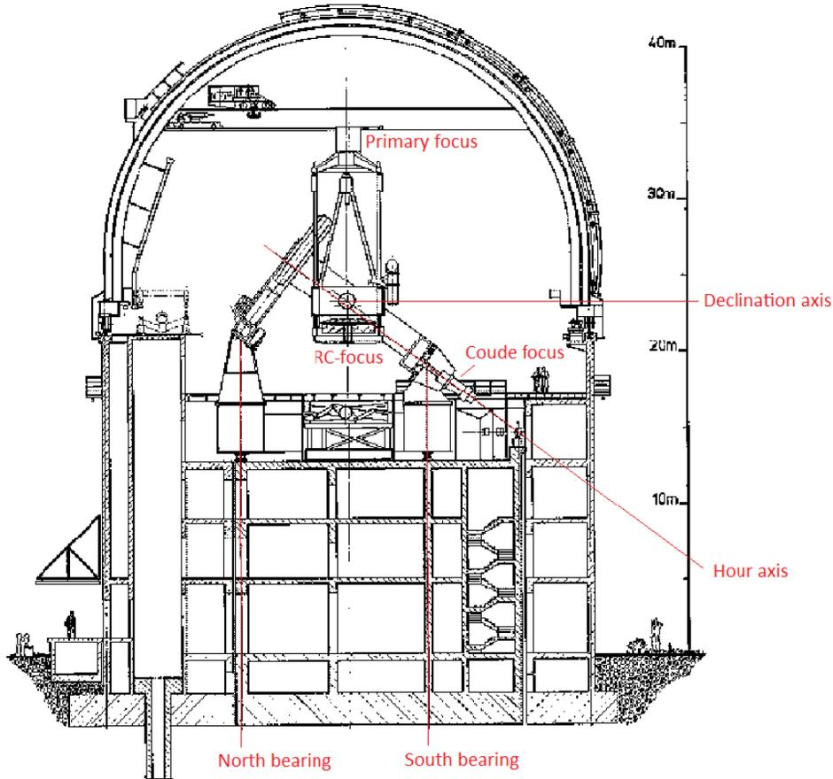
**Scheme of the Calar Alto 3.5 m telescope:** You can see the primary focus and the RC focus are independent from the declination and hour axis—they are not important for these foci. The Coudé focus on the other hand demands a number of mirrors in the cross-sections of these axis which leads to a high engineering effort.
