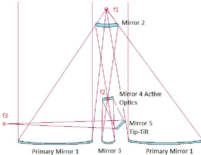
beams to two mirrors (mirror 3) which then combine the beams in the interferometer focus f4 not without passing through two lens systems and reflection by mirrors 6. The tube itself is designed for maximum rigidity and the active optic makes up for any deformation of the tube structure.
