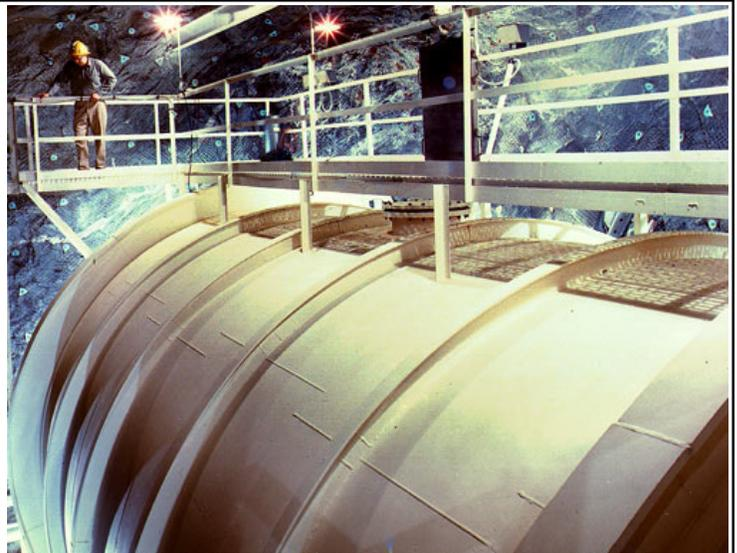
The tank filled with 100,000 gallons of tetrachloroethylene (a simple dry cleaning fluid) in the Homestake mine.
