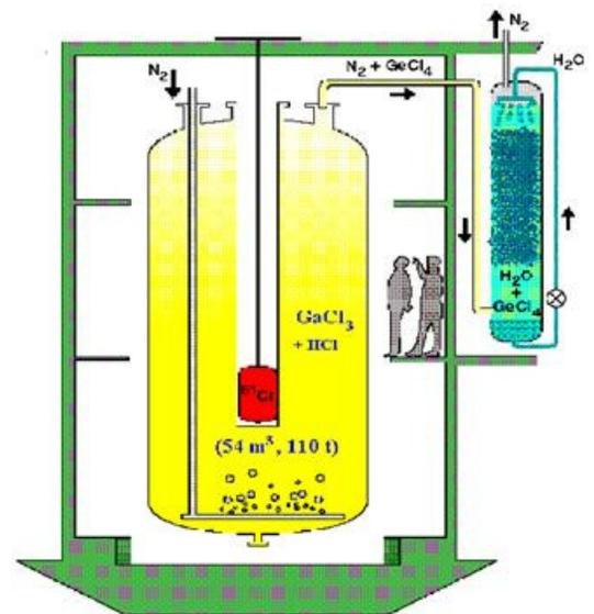
Scheme of the GALLEX experiment: By counting the radioactive atoms of germanium, the neutrino flux is calculated.
