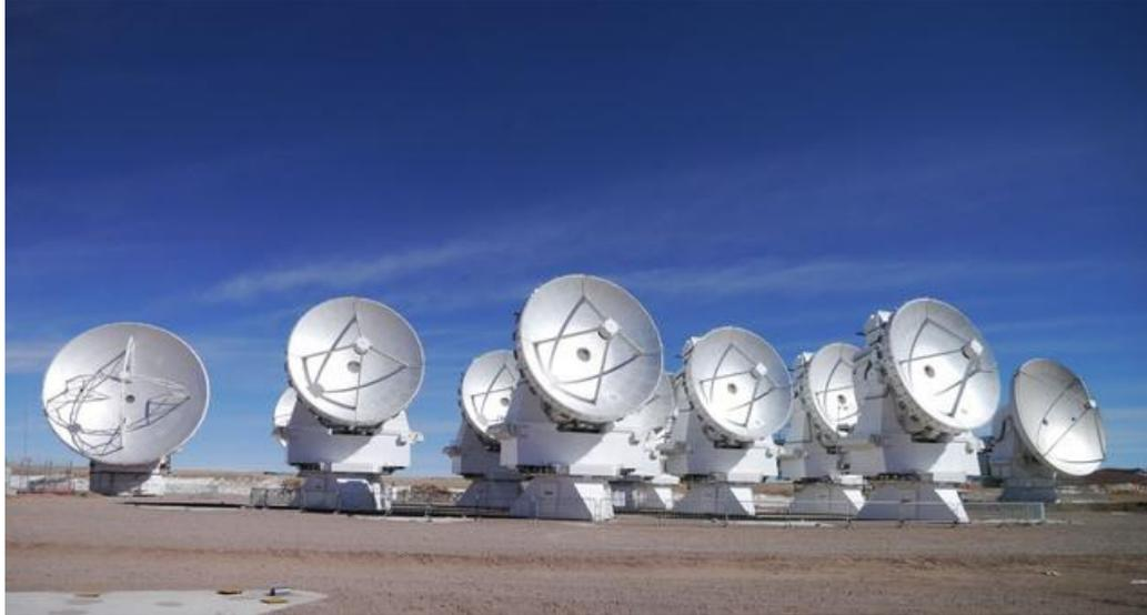
The Atacama Compact Array (ACA) is a sub-system of the ALMA telescope which allows enhanced imaging fidelity especially for extended astronomical sources. The ACA comprises of 16 (four 12-m and twelve 7-m) antennas, the last of which was delivered by Japan in May, 2012. Credit: ALMA(ESO/NAOJ/NRAO), R. Hills
